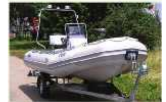
Forward view of R-470 Lux, showing deep 'V' formed in boat's hull by inflatable keel. This assures superlative handling and planing capabilities
