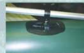
Positive rowlock location prevents oar loss
