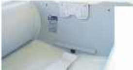
Rigid integral transom with fitted plastic plate for engine location
