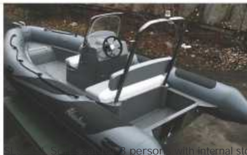
SLS-4 Soft seat for 3 persons with internal stowage and soft backrest, navigation arc and navigation lights Dimension, cm: (L x W x H) 124 x 60 x 135 Available for: V-550
